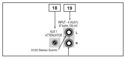
Fig. 14A - Stereo Summing and AUX 1 Input Attenuator
